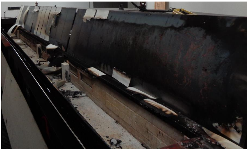
Photo No. 4 Exposed Surface of the Test Specimen (Post-test)
